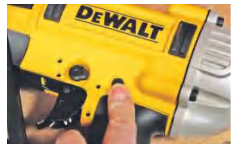
The DPN1564APP gun also has a blower function, which can be operated by pressing this button
